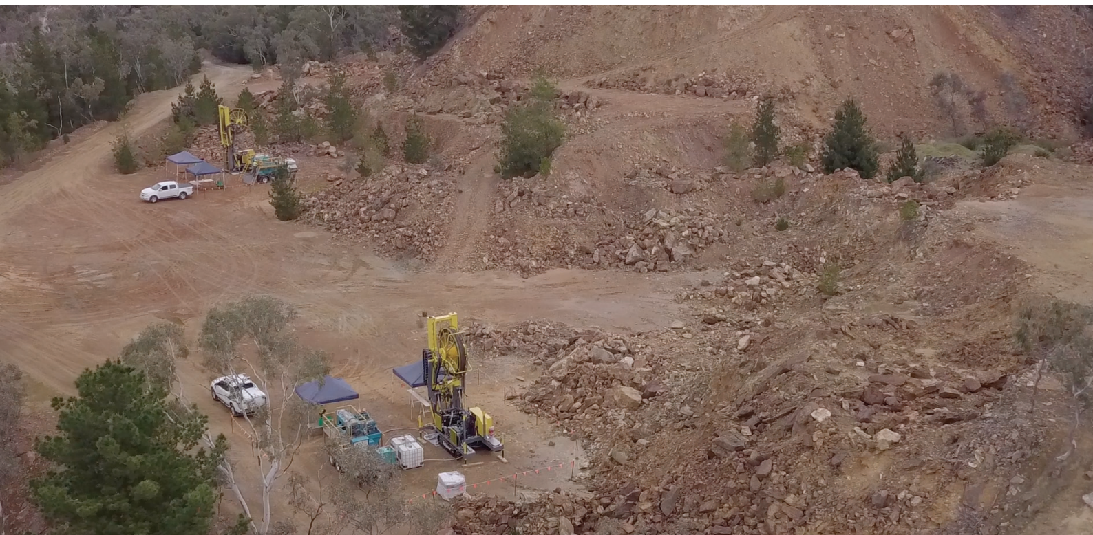
Two of the next generation RoXplorer® drill rigs in action at Brukunga (South Australia), using coiled tubing to achieve highly efficient deep penetration sampling of exploration targets. Image courtesy of Deep Exploration Technologies Cooperative Research Centre (DET CRC).
