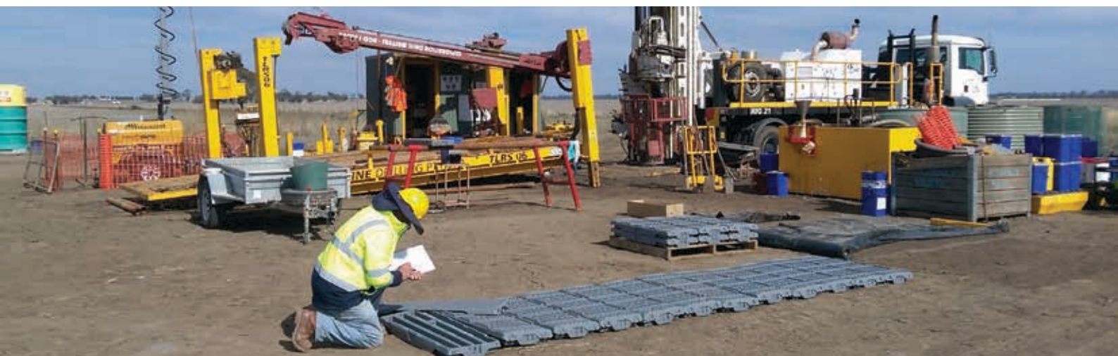
Diamond drilling into Cambrian basement through 250 metres of sediments of the Murray Basin in western Victoria. Image courtesy of Auspac Resources.
