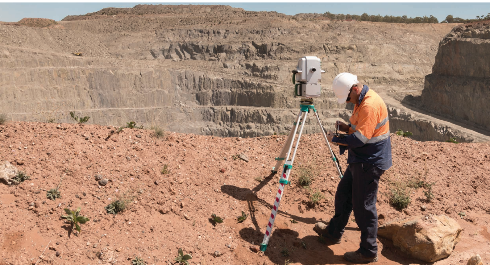
Maptek manufactures long range, lightweight 3D laser scanners for fast, accurate mine survey. A visit to the facility is offered as a field trip (FT12) during the Convention. Image courtesy of Maptek.
